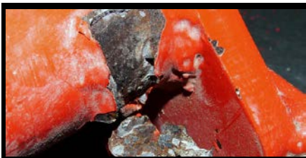
Failed scissor pack yoke
